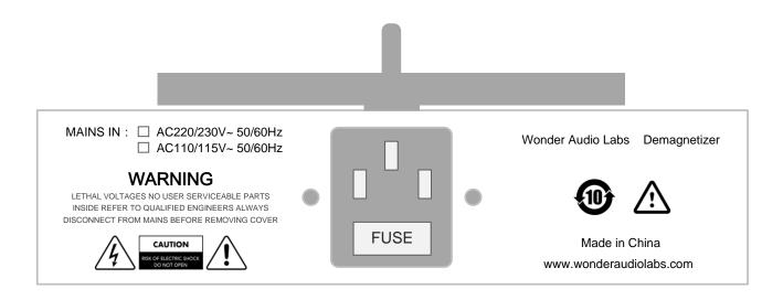
The Demagnetizer is equipped with an IEC 320 mains inlet socket. Use the supplied mains cable to connect the unit to the local mains supply. The mains fuse and a spare are located in the compartment next to the mains in on the rear panel.
